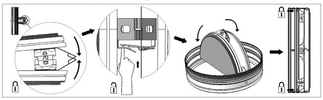
The fire damper is equipped with a spring for closing the blade: pay attention to the hands.
