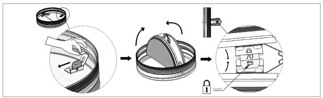
The fire damper is equipped with a spring for closing the blade: pay attention to the hands.
